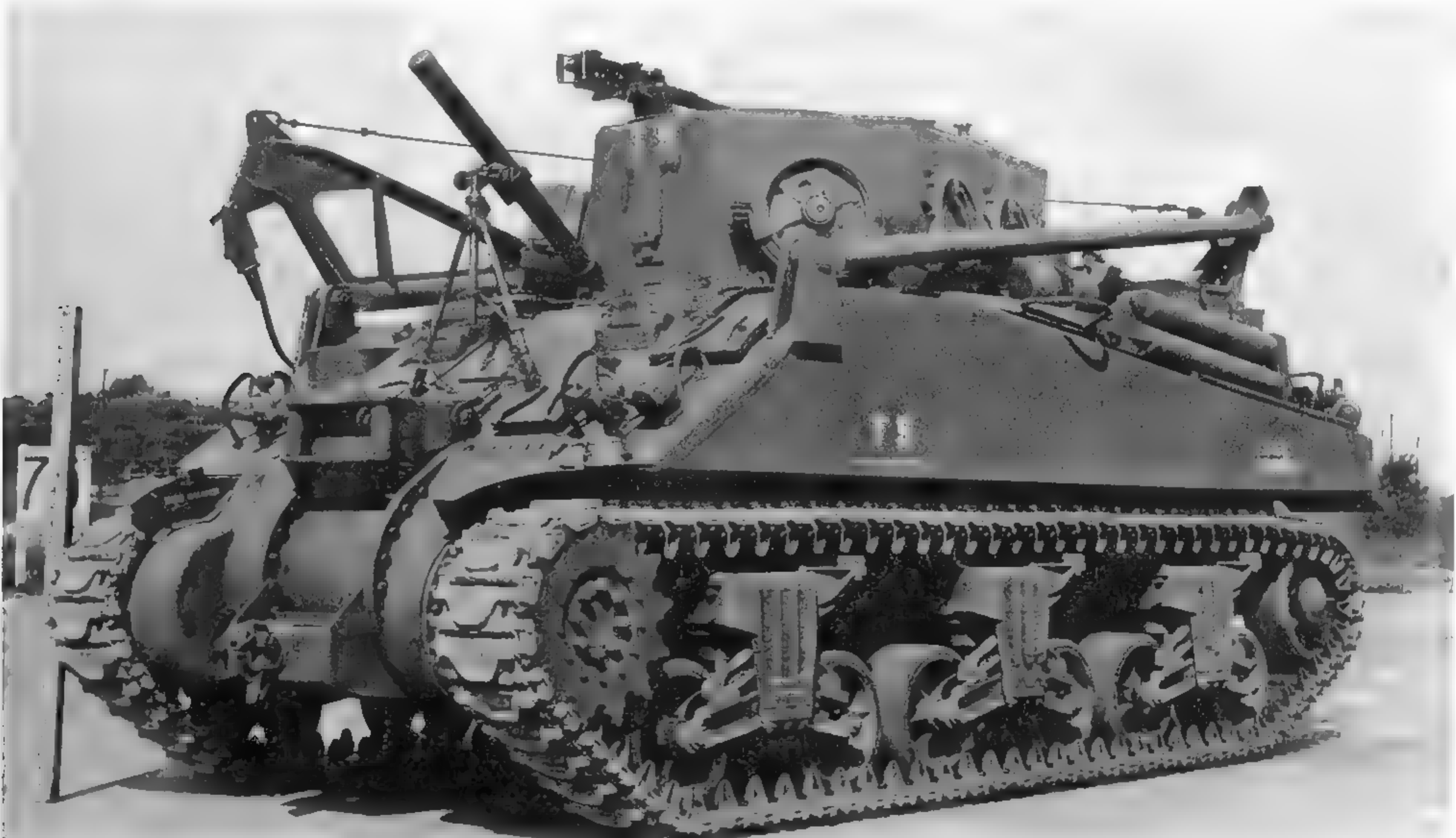
The T5 was the test model for the series that became the M32. Built by Lima Locomotive Works, this T5 was photographed at Aberdeen Proving Ground in September 1943. The production M32 varied very little from the T5. (National Archives and Records Administration photo)
